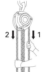
●If the hoist still fails to go into high speed after trying the above methods, lift a load greater than the lifting switch load (See P.2, ■Lifting Switch Load) and then lower it and remove the load.
