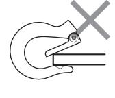
The load is applied at the tip of the hook.
