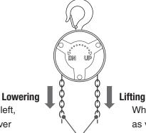
When the hand chain on the left, as viewed from the wheel cover side, is pulled down (in a DN direction), the load is lowered.
