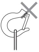
The holding object or the sling is not hooked in the correct position.
